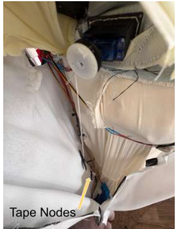
Fig. 8: A look between the bi-layer: Taped-thread stoppers positioned along lifting lines to pin fold locations and block over-travel, improving symmetry and repeatability.
