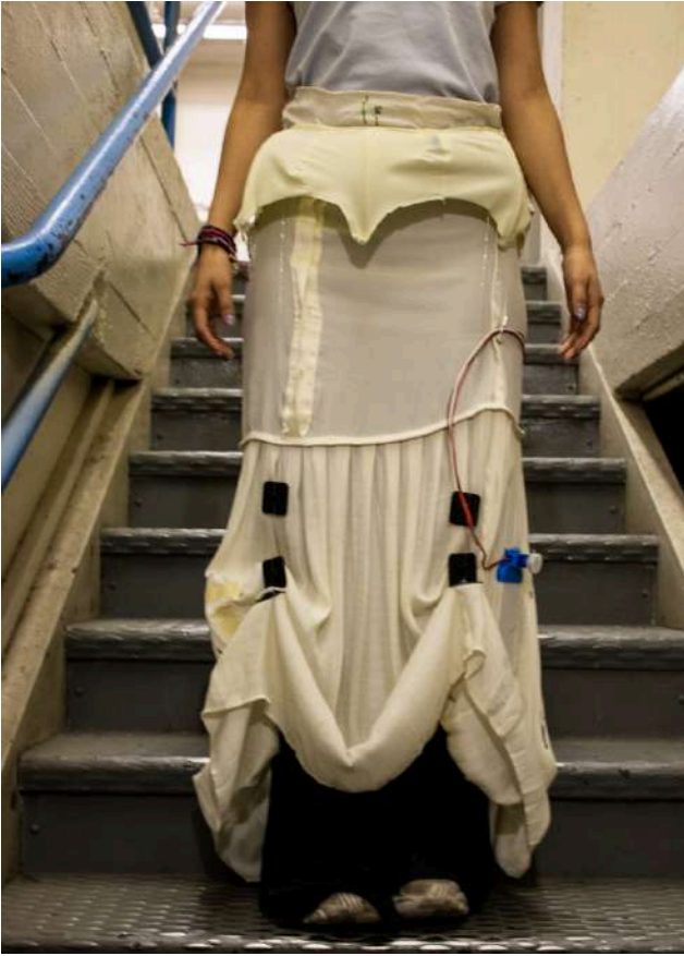
Fig. 13: Stair ascent sequence showing auto-lift activation, hem shortening, and flipper curl for toe clearance.
