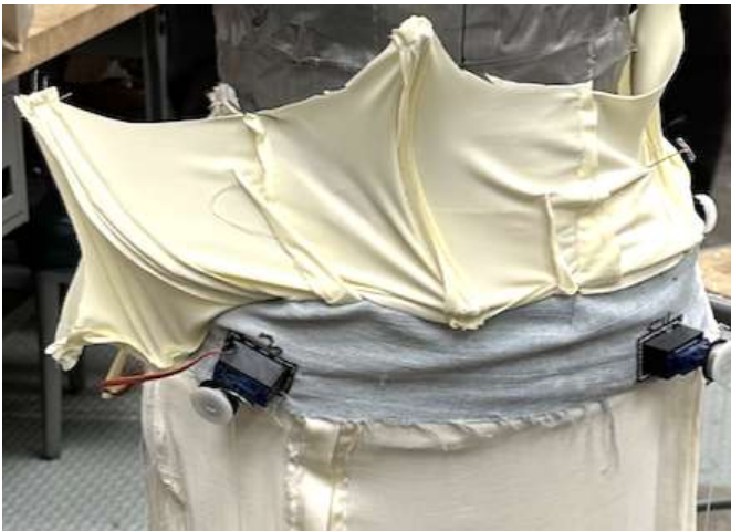
Fig. 7: Corset is flipped upright, showing motor integration and design. Motors were placed in a TPU housing and hand stitched into the base. Denim was used under the corset to provide more stability since it is stiffer and holds more weight.
